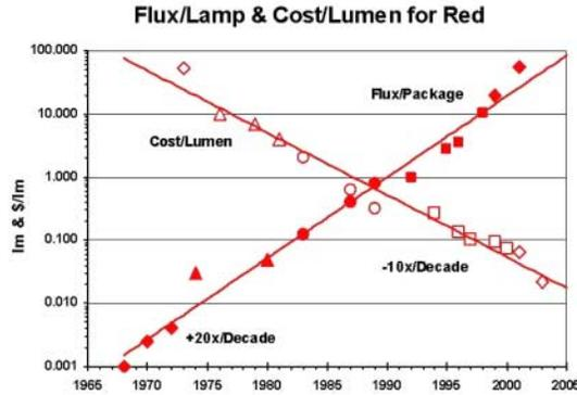
**Fig. 5.** Evolution of red LEDs over more than three decades. The line labeled “Flux/Package” represents the most powerful commercially available LED in a given year. The *line* labeled “Cost/Lumen” describes the price decline per unit of flux for the highest volume LED customers in that year
