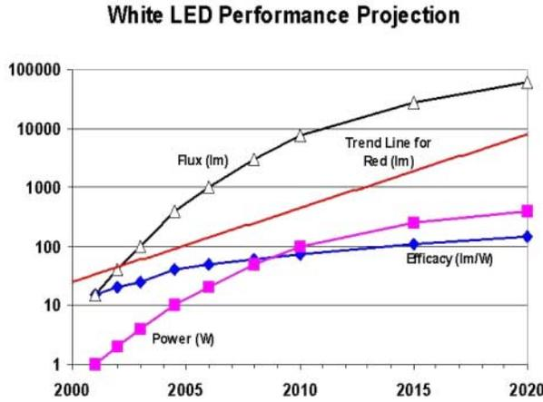
**Fig. 8.** Near term flux performance of white LEDs and extrapolation to 2020. Efficacy is expected to increase by 10× to 150 lm/W while drive power will increase by 500× to 500W in 2020. By 2010, white flux will be ahead of the red trend line by 20×
