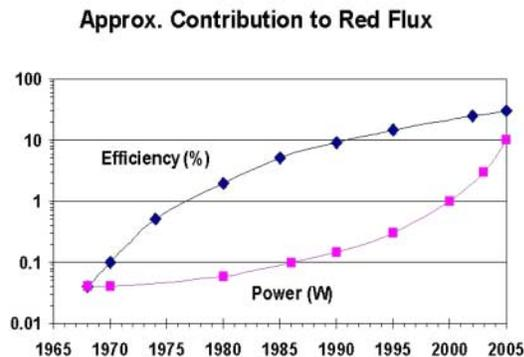
**Fig. 6.** The two main drivers of the flux trend line in Fig. 5 are efficiency and drive power. In the early years, practically all improvements are due to efficiency. In the later years, efficiency saturates and drive power becomes the dominant factor
