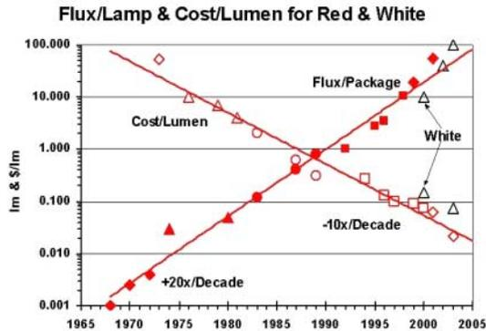
**Fig. 7.** Superposition of early white flux and cost data on the red trend lines of Fig. 5. White flux is crossing the red trend line in 2002 while cost remains a factor of  $2\times$  above the trend line
